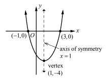
The graph of the quadratic function  $y = x^2 - 2x - 3$  opens upward since a = 1 > 0, so the vertex is a minimum point. The equation of the axis of symmetry is  $x = -\frac{-2}{2(1)}$  or x = 1.
